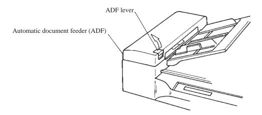
Figure 5.1 Removing jammed documents
